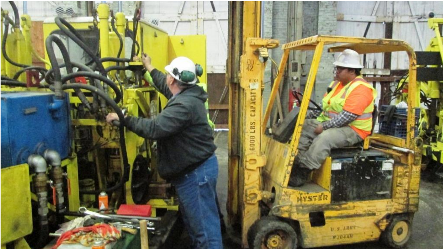
Chris and Alan attach a sling to the cylinder guide as Anthony on the forklift lifts it out of the tie-shear
