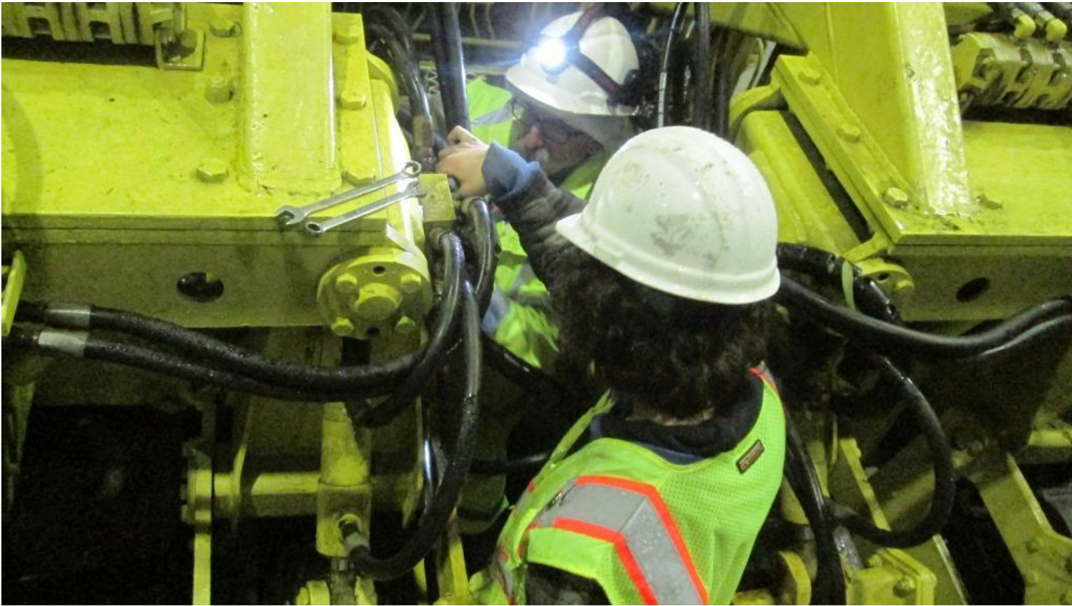
Now in the Erecting Shop where conditions are better, Joe and Matt begin removing the vibrator motor
