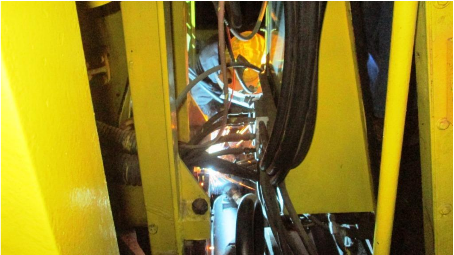
Cliff welds new latch-hooks to the tie-shear's kicker
