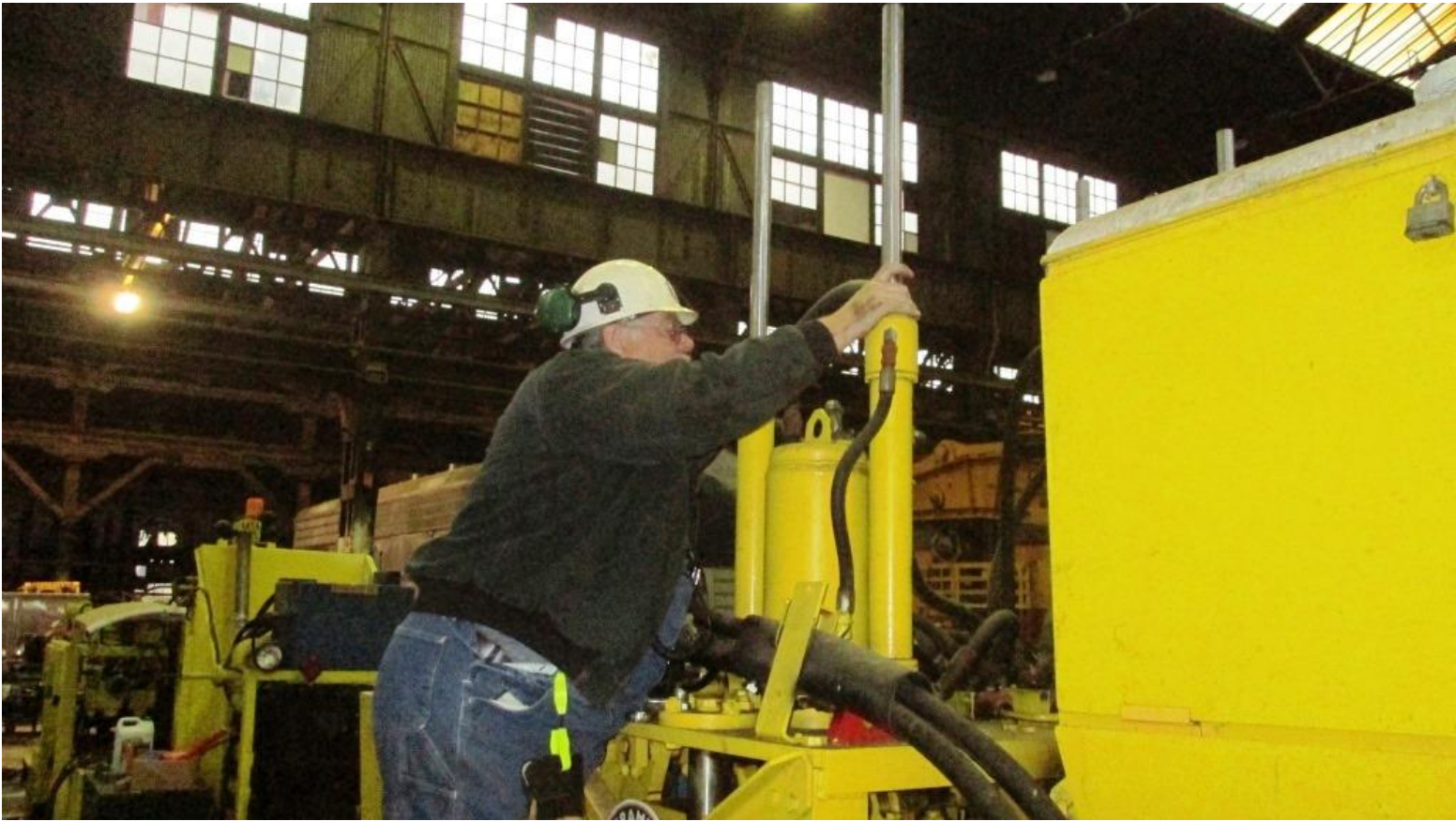
Chris begins the process of disassembling the main lift-cylinder for the shear
